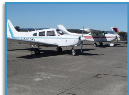
Tie-down Apron: Spaces for based and smaller transient aircraft are normally equipped with tie-down anchors and chains or ropes to prevent the aircraft from being blown around by
