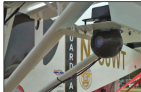
CH 750 "Guardian" equipped with pan-tilt-zoom camera - ideal for fire watch and SAR
