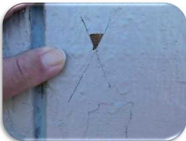
Figure 5-59 shows the results of an adhesion test indicating poor adhesion.
