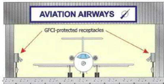
Figure 7-3. GFCI protection is required for 125-volt, single-phase, 15- and 20-ampere receptacles operating at 50/60 hertz.
