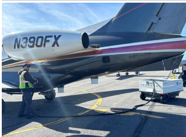
Alan connecting new Zero Emissions eGPU for the first time.
