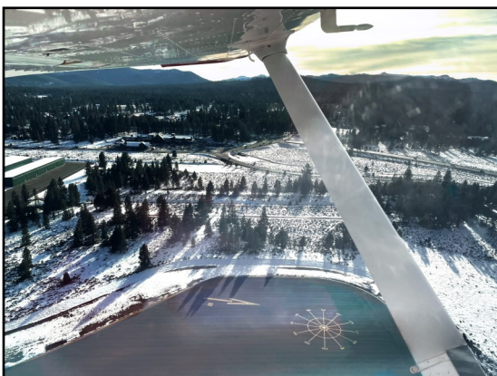
11 Runup area markings guide pilots to bypass bridge
