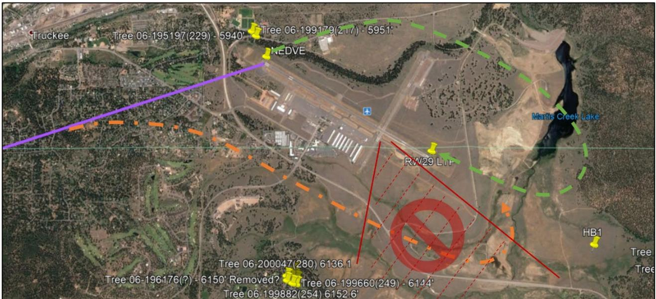
Figure 7: RNAV (GPS)-A Visual Circling path
