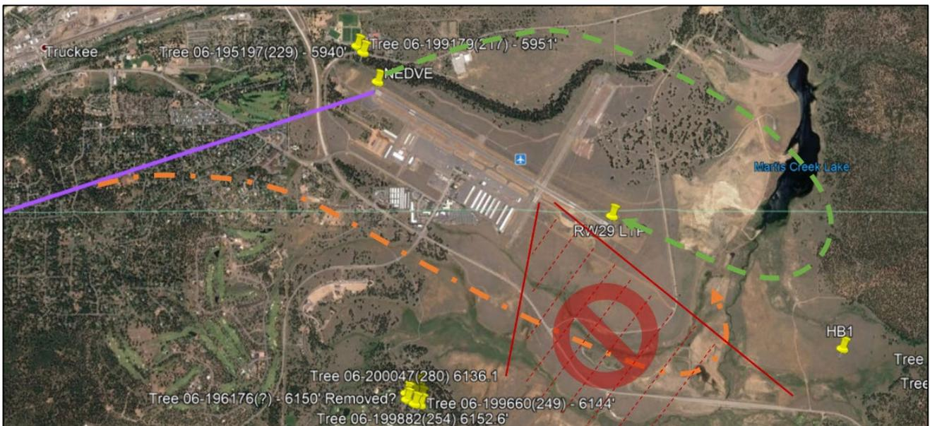
Figure 7: RNAV (GPS)-A Visual Circling path
