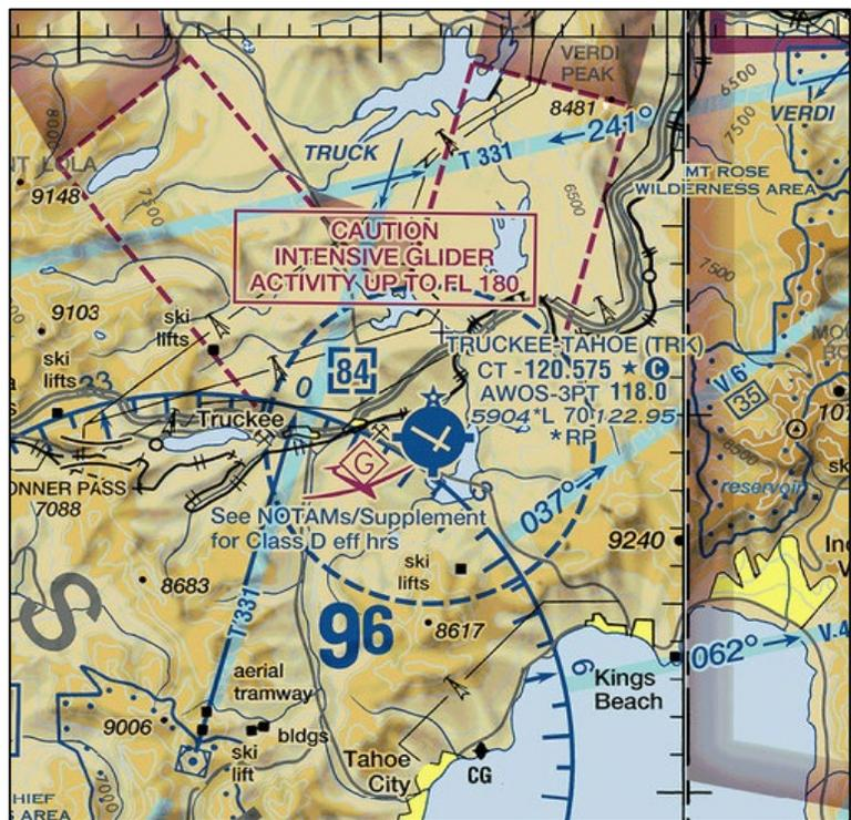
Figure 1: TRK Airspace Diagram
