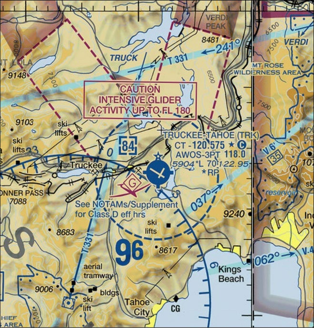
Figure 2: TRK Airspace Diagram
