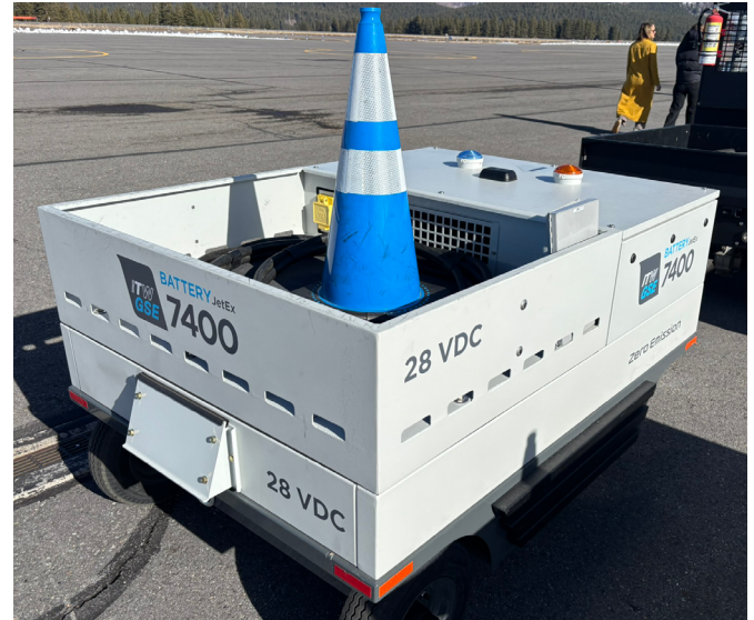
"Electric ground power units (eGPUs) provide aircraft with power before the engines start"
