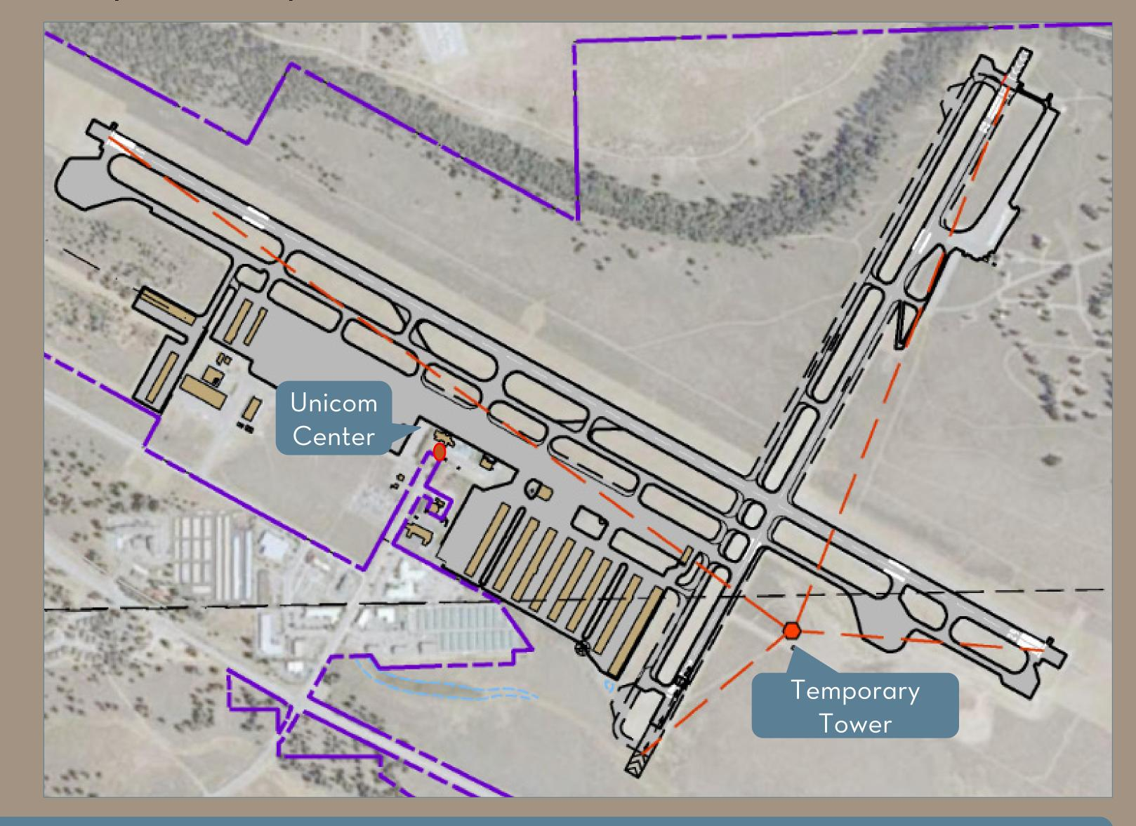
Step II: Establish a temporary Tower (mobile unit) with view of all runway ends
