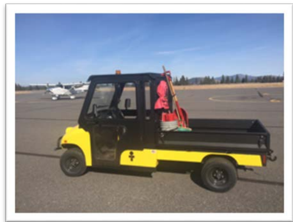
New Columbia Car Electric Ramp Truck purchased in 2018 to replace gas powered Kawasaki Mules.
